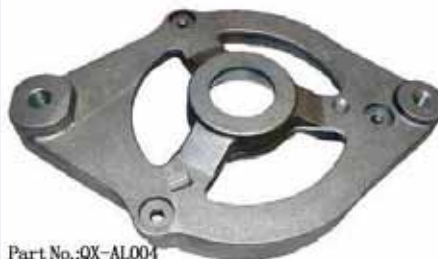
Part No.: QX-AL004 Description: ID: 127mm Bearing Bore Dia: 40mm Foot to Bearing Center: R90.5 Φ10 R85 M8
