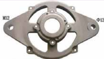
Part No.: QX-AL330 Description: ID: 138mm Bearing Bore Dia: 62mm Foot to Bearing Center: 2-R99 M12X1.25 Φ13
