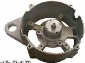
Part No.: QX-AL331 Description: ID: 138mm Bearing Bore Dia: 35mm Foot to Bearing Center: R99 Φ22
