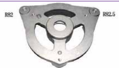
Part No.: QX-AL066 Description: ID: 113mm Bearing Bore Dia: 42mm Foot to Bearing Center: R82 R82.5 2-Φ8.5
